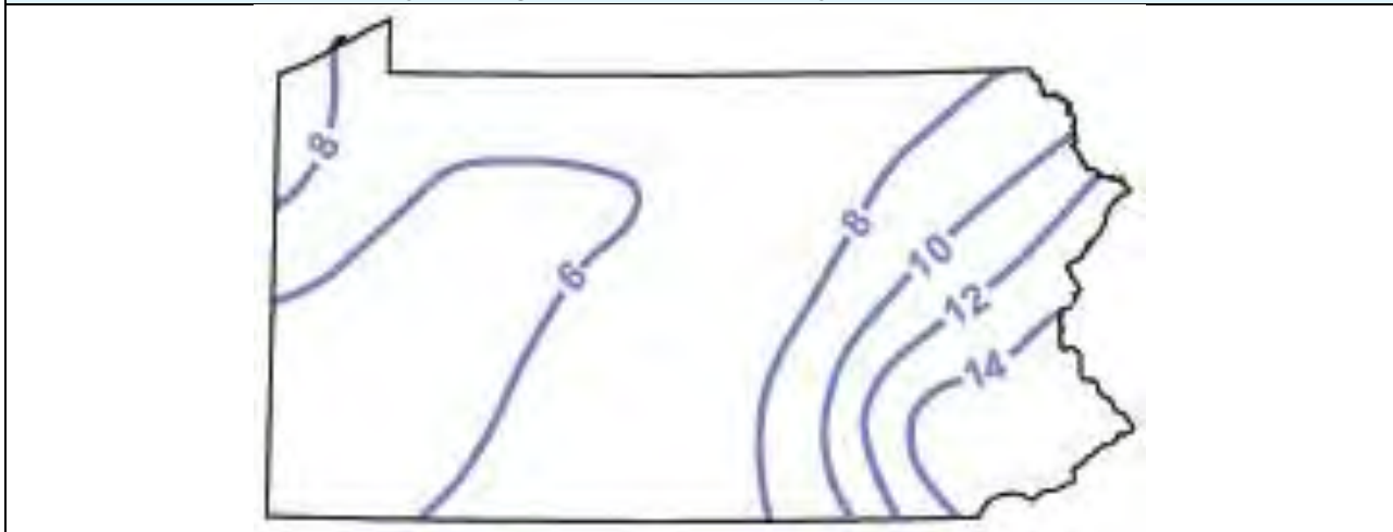
Figure 4.3.3-6 Pennsylvania probabilistic earthquake hazard map. Contours represent PHGA values that have a 2-percent probability of being experienced over a 50-year period (PADCNR, 2007).
